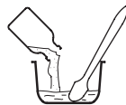
Add tobramycin powder to STIMULAN Rapid Cure powder and mix for 30 secs
