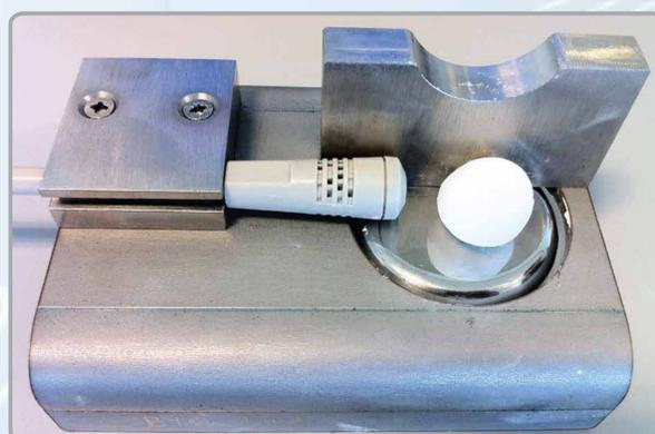
Figure 5. Apparatus used containing microphone, plate and sample drop height guide
